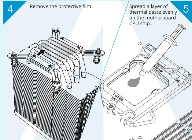
Spread a layer of thermal paste evenly on the motherboard CPU chip.
